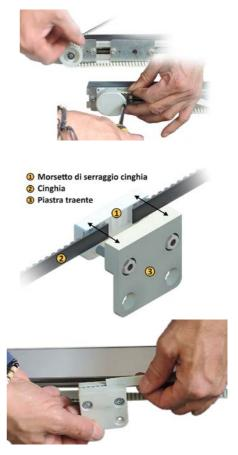
The pulling plate acts as a joint between the two edges of the belt and when suitably fixed, as well as ensuring the perfect tightening of the belt, it transmits the movement of the belt to the door.
