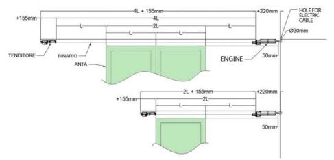
Actuator can be positioned to the right or left - All measurements are to be considered in millimeters, mm.
